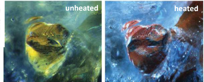
Figure 2. Left: This Sri Lankan sapphire hosts a blocky iron sulfide inclusion with a surface-reaching crack, both of which are coated with yellow limonite. Right: After heating in air to 350°C, the limonite coating on both the sulfide and the related fracture changed to rust-colored hematite. Photomicrographs by J.J. Koivula, magnified 10x.
