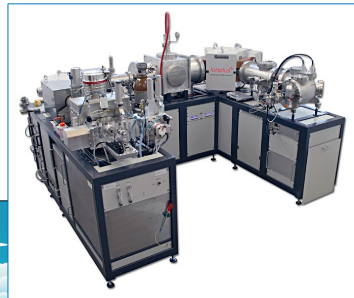
MICADAS Mini Carbon Dating System (Accelerator Mass Spectrometer). Image ETH Zurich & ionplus AG
