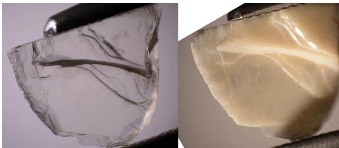
Figure 5. The colorless diasporite fragment (sample 97003) before heating (left), transformed to whitish corundum with tiny micro-fissures after dehydration (right). Image width 10 mm.
