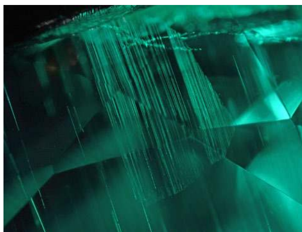
Figure 14: Fine parallel hollow tubes along the c -axis are present in this Musakashi emerald. Photomicrograph by M. S. Krzemnicki, © SSEF; magnified 50 \times .
