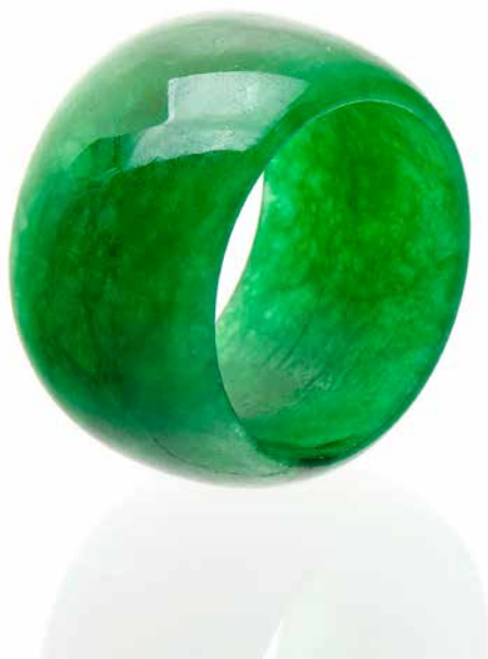
△ Figure 1: Treated jadeite-jade (polymer impregnated and dyed). Photo: L. Phan, SSEF.
