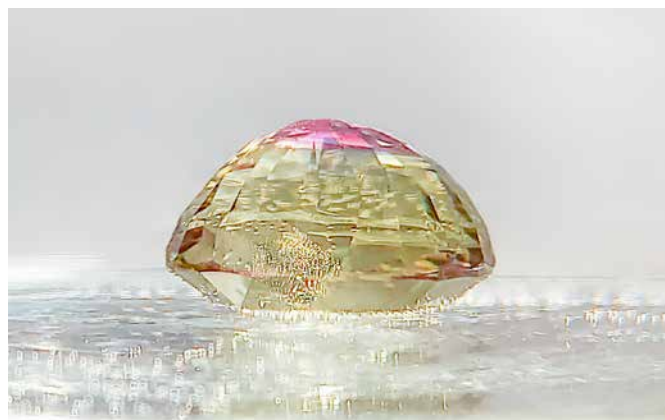
△ Figure 3: Distinct chromium-rich zonation at the culet showing a red colour when observed with an incandescent light source. The stone was immersed in water to minimise reflections. Photo: P. Lefèvre, SSEF
