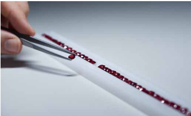
△ A comparison of ruby colour under standardized lighting conditions in the SSEF light box. Photo: SSEF.
