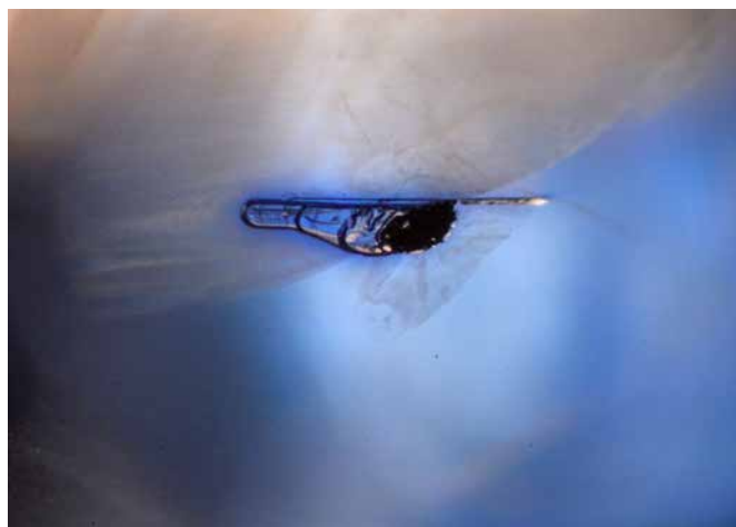
△ Figure 3: Diffused blue zone and dark blue spot around small cavity filled with glassy residue in one of the Ti-diffusion treated sapphire cabochons. Photo: M.S. Krzemnicki, SSEF.
