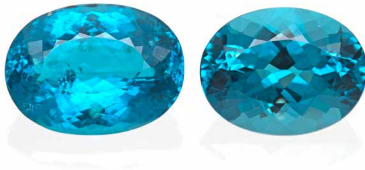
△ Figure 1: Submitted as a matching pair of Paraiba tourmalines, our testing revealed that only the left stone is copper-bearing, whereas the right stone was identified as an indicolite tourmaline. Photo: L. Phan, SSEF.
