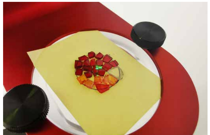
△ Figure 2: Research samples after a gamma irradiation experiment carried out by SSEF. The rubies used for this experiment have not really changed their colour, whereas the originally pink sapphires have become distinctly orange. Photo: H.A.O. Wang, SSEF.
