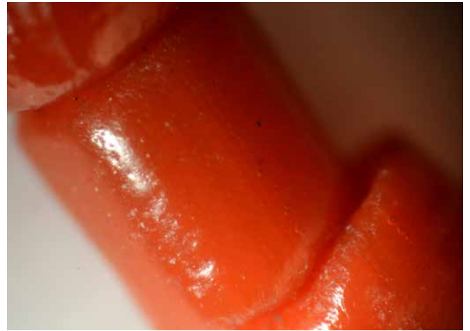
△ Figure 2: Distinct air bubbles in glass beads imitating a coral necklace. Microphoto (50x magnification): M.S. Krzemnicki, SSEF
