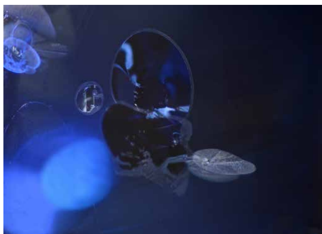
△ Figure 2: Disc-like extension features in one of the described cabochons as proof of heating at high temperatures during the Ti-diffusion treatment. Photo: M.S. Krzemnicki, SSEF.
