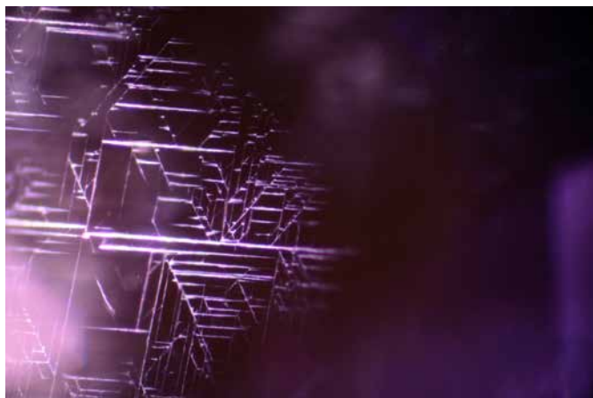
△ Figure 2: Oriented needle-like inclusions in the described hackmanite. Photo: M.S. Krzemnicki, SSEF.
