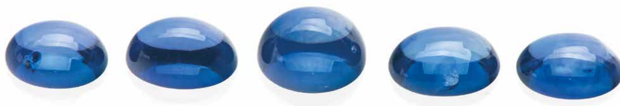
△ Figure 1: Five Ti-diffusion treated sapphires examined at SSEF. Photo: SSEF.
