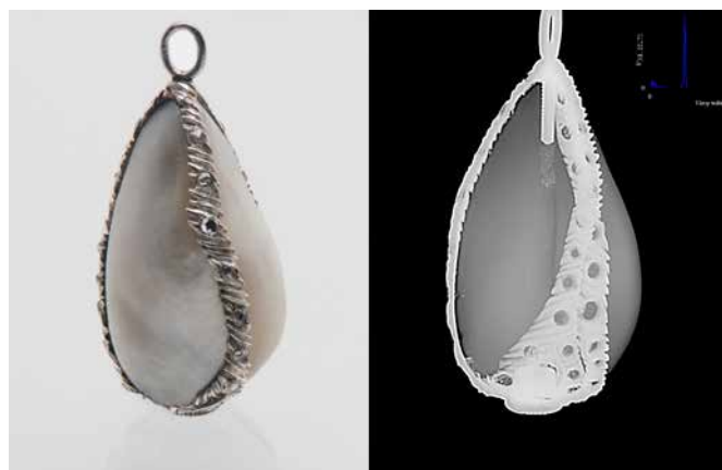
△ Figure 3: Pendant made of three curved shell pieces and radiography showing two of these pieces with a grey vertical intersection line where these two parts were glued together. Photo: SSEF.
