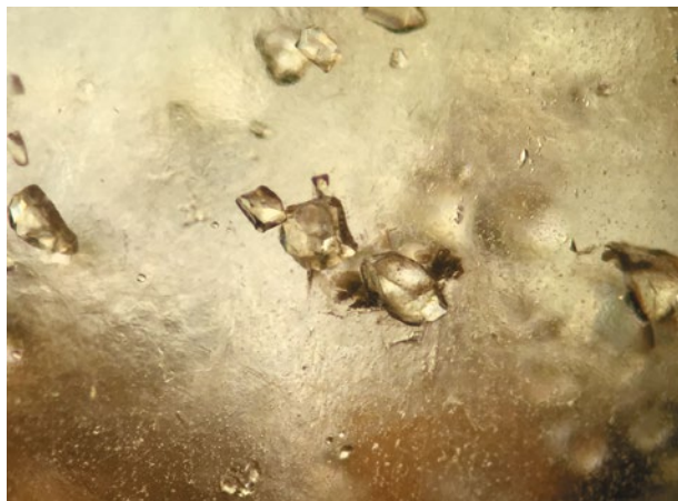
Figure 9: Raman analysis identified this group of well-formed crystals as titanite. Photomicrograph by S. Hänsel; image width 2.8 mm.
