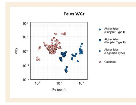
Figure 15: This plot of Fe vs V/Cr (based on LA-ICP-TOF-MS data) reveals that Afghan emeralds—and specifically Panjshir type II material—can be separated from Colombian emeralds. The Fe concentration in Panjshir type II emeralds is generally higher than in Colombian emeralds, except for a few 'Fe-rich' Colombian stones. By plotting Fe against the V/Cr ratio, however, even these 'Fe-rich' Colombian emeralds can also be clearly separated from Panjshir type II material.
