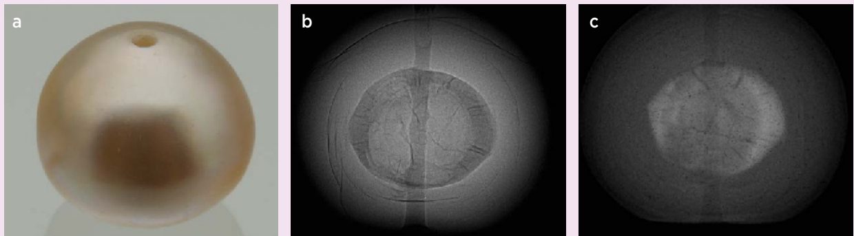
Figure 3: (a) Saltwater natural pearl NP-2e ( Pinctada radiata , 10.3 mm in diameter) is shown here with its X-ray radiograph (b) and neutron radiograph (c). The inverse attenuation of the organic-rich core (dark grey in X-rays and light grey in neutrons) and the dense surrounding nacre layer (light grey in X-rays and dark grey in neutrons) is obvious.
