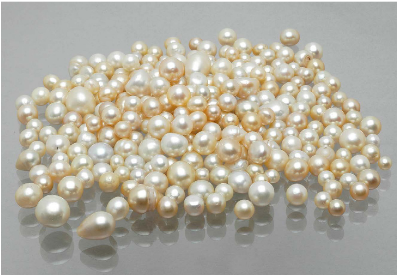
Figure 1: These pearls (0.7–9.3 ct) were submitted to SSEF for identification and differentiation into natural or cultured origin. Neutron imaging can complement the use of X-rays for difficult cases of identification that might be encountered in a group of pearls such as this. Photo by Luc Phan, © SSEF.
