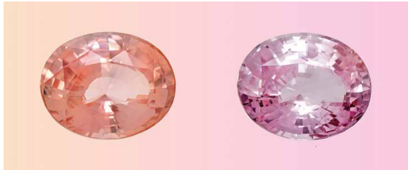
Figure 1: Fancy sapphire recently found in Madagascar showing an unstable color, shifting from pinkish orange (padparadscha-like) to pink after a fading test. (Photo: SSEF)
