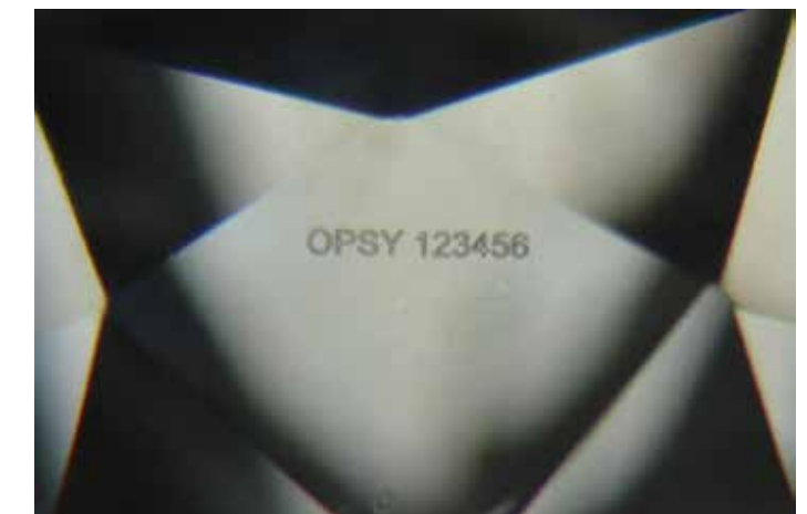
Figure 3: Sub-surface inscriptions in diamonds with the Opsydia D5000 Diamond Marking System. Left: low intensity mark within the diamond's table not viewable through a loupe. Right: larger loupe-readable mark in a star facet. Bottom: large loupe-readable logo mark. (Photos: Opsydia)
