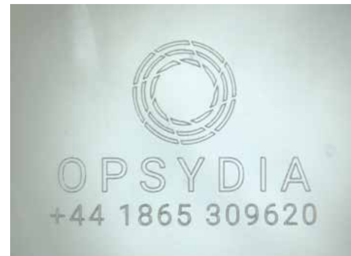
Figure 3: Sub-surface inscriptions in diamonds with the Opsydia D5000 Diamond Marking System. Left: low intensity mark within the diamond's table not viewable through a loupe. Right: larger loupe-readable mark in a star facet. Bottom: large loupe-readable logo mark. (Photos: Opsydia)
