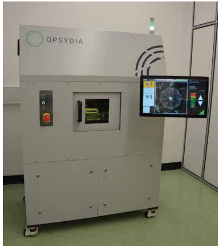
Figure 4: Opsydia sub-surface diamond marking system. (Photo: Opsydia)
