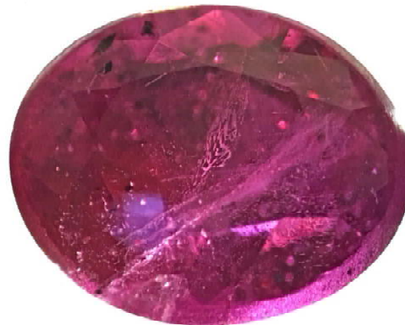
Knischka Synthetic Ruby with Flux Residue
