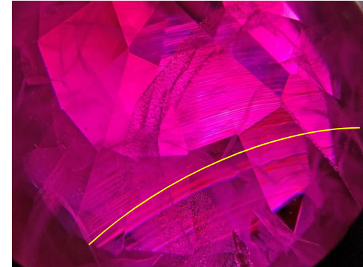
Cracked Synthetic Verneuil Ruby Heated with Flux
