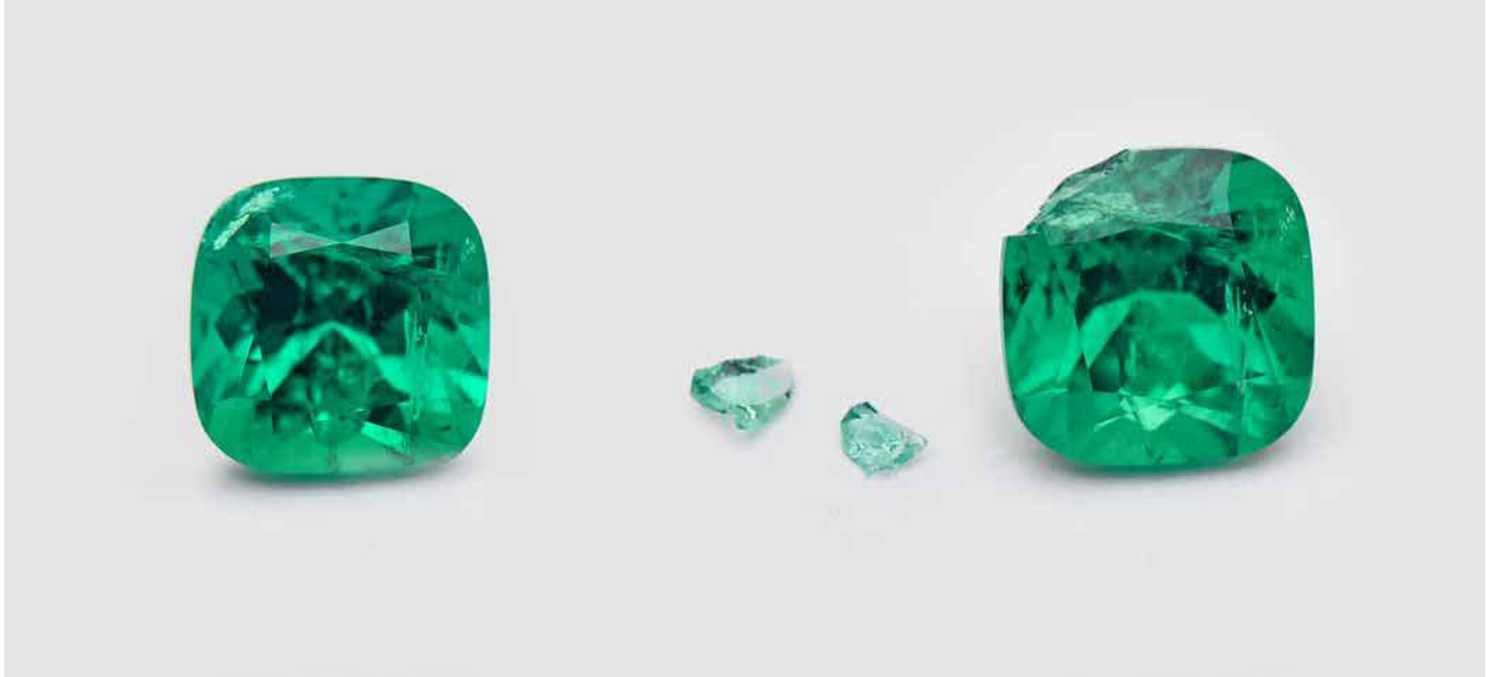
△ Figure 1: Before and after photos of an emerald with an evident (cleaned) fissure in the upper left corner, which spontaneously chipped at SSEF during normal testing procedures. Photo: V. Lanzafame, SSEF
