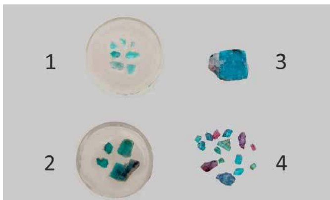
△ Figure 5: Prepared Paraíba tourmaline samples for GemTOF analysis. (1-2) small samples embedded in epoxy-resin; (3) polished rough sample with host pegmatite; (4) polished small sample fragments of various colours. Photo: V. Lanzafame, SSEF
