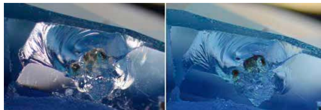
△ Figure 3: Close up (in reflected and transmitted light) of laser damage on a sapphire, showing a large chipped area (approx. 3 mm wide) at the surface produced by heat induced tension by the laser. As a further consequence, the central part has melted to finally remain as a greenish and crackled glassy residue in the laser hole. This glassy residue is best seen in the microphoto on the right side. Microphotos: M.S. Krzemnicki, SSEF
