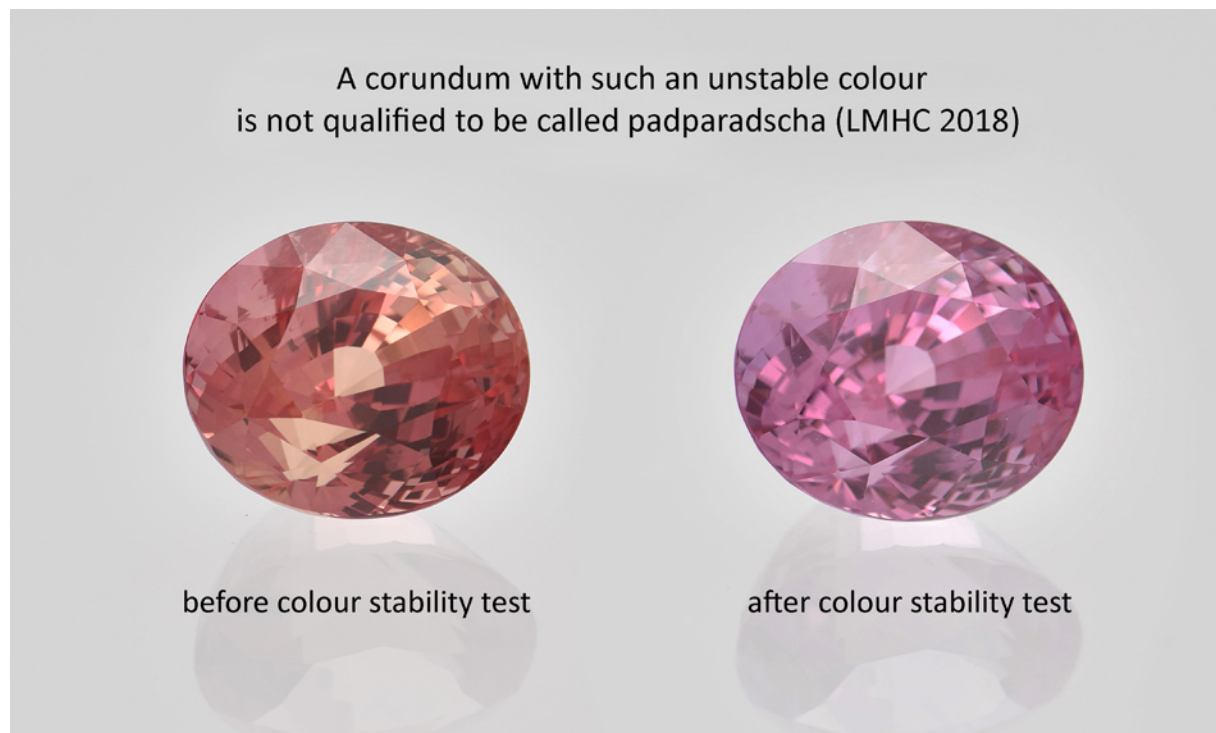
Figure 1: Corundum with unstable colour not qualified to be called ‘padparadscha’ (see modified LMHC information sheet No. 4).
