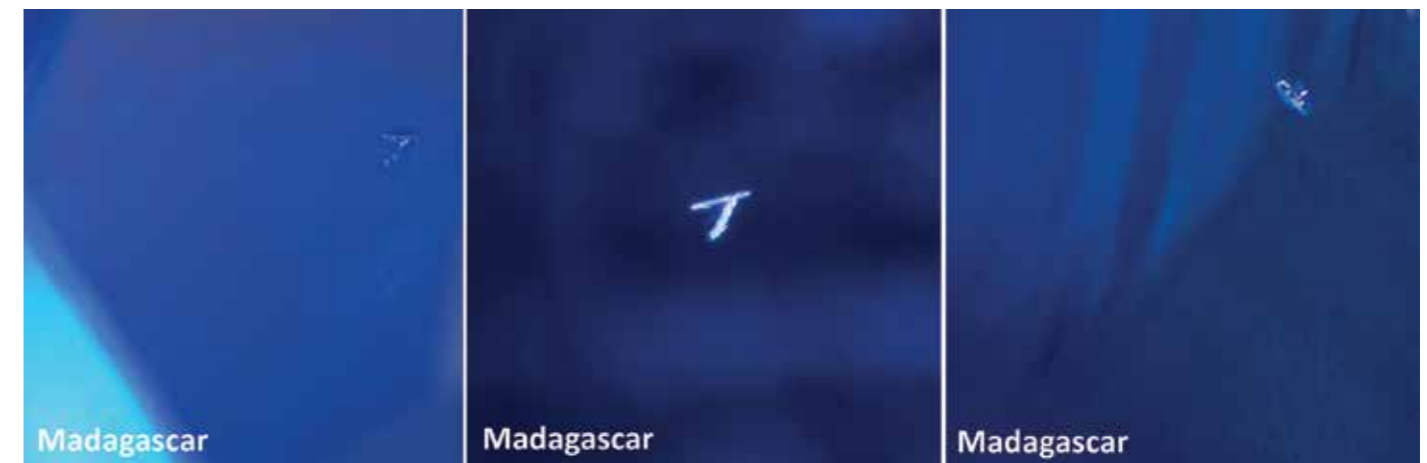
Figure 7. Tiny prismatic zircons in “Kashmir-like” sapphires from Bemainty. Magnification 50-70X. (Photos: M.S. Krzemnicki, SSEF)
