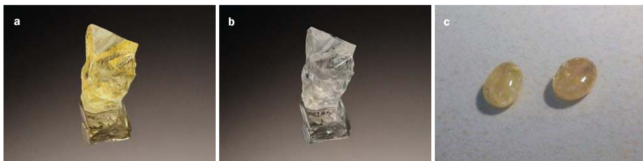
Figure 8: A rough yellow danburite from Namalulu, Tanzania, (a) was heated to 500 °C for four hours, resulting in a complete loss of colour, and the sample remained colourless after further heating to 950 °C for 24 hours (b). For another test, one bead of Namalulu danburite was kept as a reference sample, while another bead was exposed to a tensor lamp for eight hours (c, left and right samples, respectively). After three hours, the bead exposed to the lamp darkened and became more brownish. Photos by Bilal Mahmood (a, b) and C. P. Smith (c).
