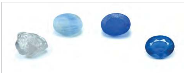
Figure 1. Series of spinels before (2 samples on the left) and after diffusion-treatment with Co (two samples on the right).
