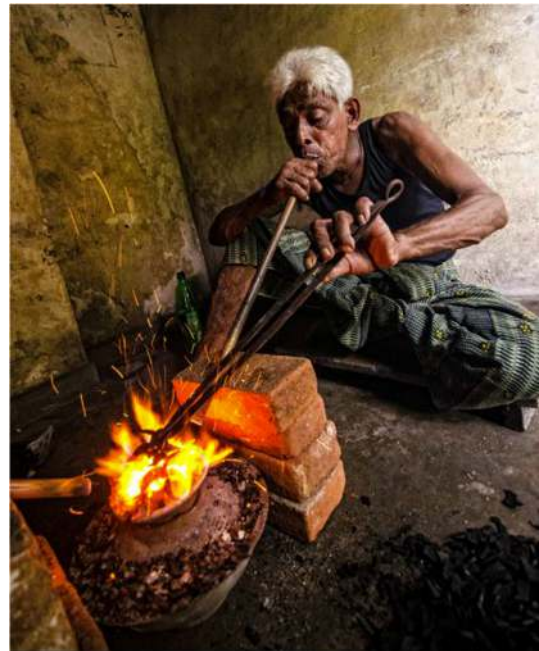
Figure 4. Traditional heat treatment of gemstones in Ratnapura, Sri Lanka. Photo courtesy of Richard W. Hughes/Lotus Gemology.
