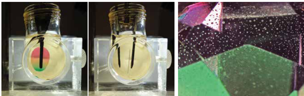
Figure 18: Left: A quartz doublet imitating bicoloured tourmaline (8.37 ct; no. 14) is shown immersed in benzyl benzoate, in views both perpendicular (left side) and parallel (right side) to the girdle plane. Right: The bicoloured tourmaline imitation contains a more concentrated area of gas bubbles near the girdle area (image width ~5 mm). Photos by H. A. Hänni.
