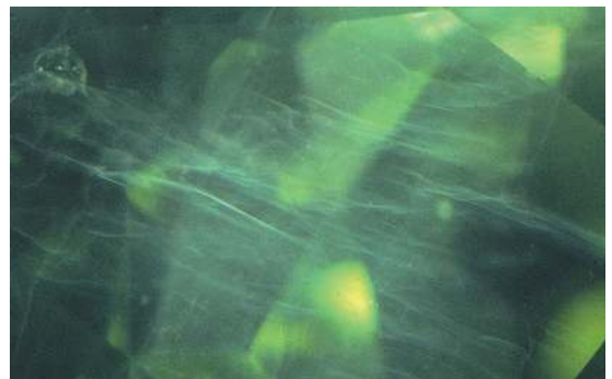
Fig. 5 Milky veils, probably a transition from olivine to serpentine in a peridot from Myanmar. Width of image 2.5 mm. Photo © H.A.Hänni
