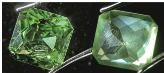
Fig. 7 A faceted peridot before and after a bath in warm sulphuric acid. Photo © H.A.Hänni
