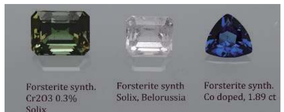
Fig. 6 Synthetic forsterites produced by Solix, Belarus. Stone on left is 12 mm long. The Cobalt blue sample is sold as an imitation of Tanzanite. Photo © H.A.Hänni
