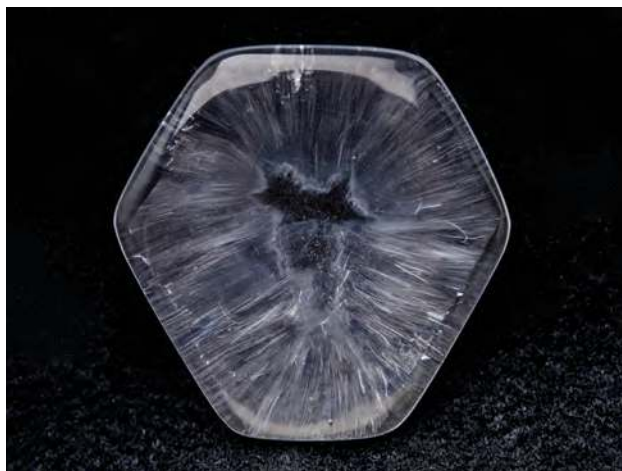
Figure 21: This 25.18 ct tablet of quartz shows a fine radiating fibrous structure (top), which is particularly noticeable when viewed between crossed polarizers (bottom). Gift of German Salazar; photos © L. Phan, SSEF (top) and by B. M. Laurs (bottom).
