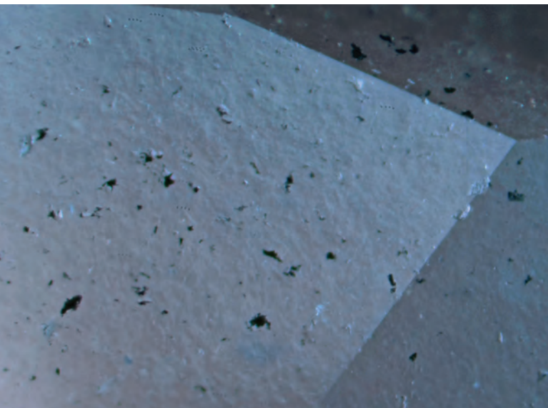
Figure 17: Viewed with the microscope, the faceted polycrystalline kyanite showed a treacle-like appearance and numerous black residues of polishing powder in small cavities on the polished surface. Photomicrograph © M. S. Krzemnicki, SSEF; magnified 60×.
