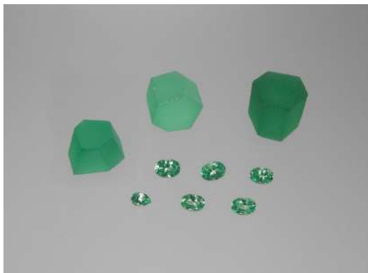
Figure 1. Rough and faceted vanadium-bearing synthetic chrysoberyls produced by Kyocera in Japan in daylight; size of the rough crystal above right 15.5 x 14.5 x 15.5 mm, weight 52.50 ct, the faceted sample below left weighs 0.49 ct and measures 6.0 x 4.0 mm. Photo by K. Schmetzer.
