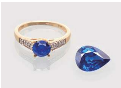
Fig. 1 These two blue imitations of sapphire are cobalt-doped cubic zirconia ( ZrO_2 ) and were tested recently at the Swiss Gemmological Institute SSEF.
