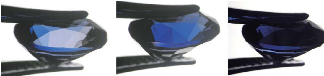
Fig. 5 Blue dumortierite in different orientations showing distinct pleochroism from near colourless to dark blue. Photo © M.S. Krzemnicki, SSEF
