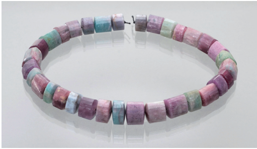
Fig. 1 Necklace with thirty-three polished beads, sold as Paraiba tourmaline proved to be a complex intergrowth of Paraiba tourmaline with lepidolite. About a third of the beads were identified as lepidolite only, showing purple colour and rather dull lustre.
