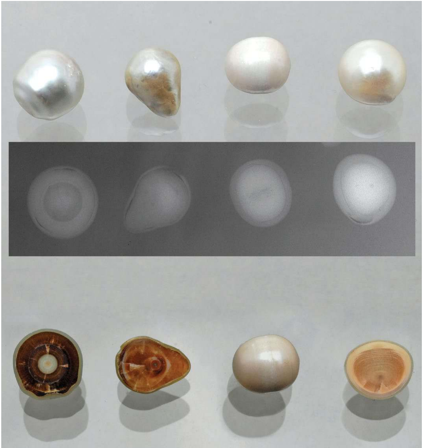
Figure 12. Four natural pearls with different shape and appearance were used as beads in P. maxima oysters. Upper row shows the coated pearls, middle row shows x-ray pictures, and lower row shows 3 cross sections. Photo © H.A. Hänni, SSEF and GemExpert.
