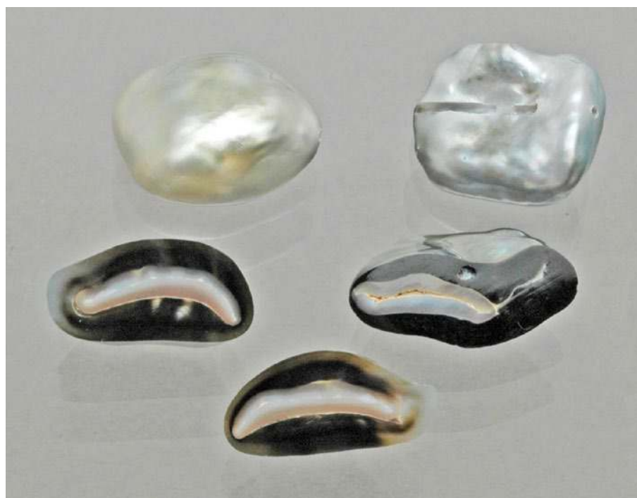
Figure 11. Beadless freshwater cultured pearls from China with a flat irregular shape are used as beads for producing baroque P. margaritifera pearls. Upper samples are shown as grown, lower samples are cut open and polished; they reveal the core of freshwater nacre. Photo © H.A. Hänni, SSEF and GemExpert.
