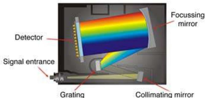
The AvaSpec-2048 is especially suitable for low light level and high resolution applications. An optional detector coating enhances the CCD performance for the UV range and a detector collection lens offers high sensitivity.
