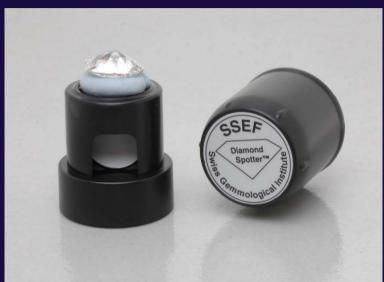
Place the diamond as shown on the diagram above, so that the SWUV light enters the diamond from a pavillion main and exits the diamond from an opposite crown main facet.
