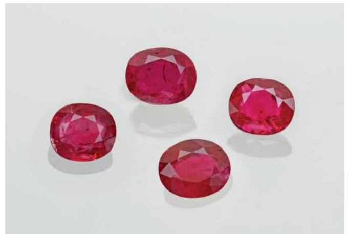
△ Figure 1: Series of rubies (2.5 - 4.5 ct) all containing fissures filled with artificial resin. Photo: V. Lanzafame, SSEF
