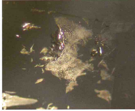
Figure 40. The presence in corundum of a white, sugary crystal with an associated stress fracture (left) is typically associated with high-temperature heat treatment. Surface-reaching fingerprint-like inclusions (right) are further evidence of heat treatment. Photomicrographs by G. Choudhary; magnified 80× (left) and 60× (right).
