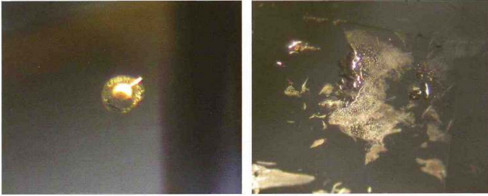
Figure 40. The presence in corundum of a white, sugary crystal with an associated stress fracture (left) is typically associated with high-temperature heat treatment. Surface-reaching fingerprint-like inclusions (right) are further evidence of heat treatment. Photomicrographs by G. Choudhary; magnified 80× (left) and 60× (right).
