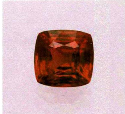
*Fig 1: Flux synthetic spinel of high purity and well-saturated colour.
