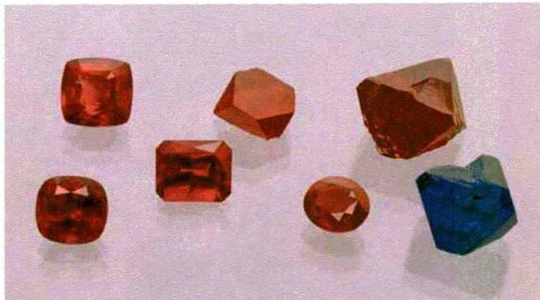
*Fig. 2: Faceted and rough flux synthetic spinels. The octahedral crystals have been produced in Russia in the early 90ies. The colour of the blue crystal is due to cobalt. Although not seen this time in the market, blue flux synthetic spinels may also appear again in the trade. © M.S. Krzemnicki, SSEF 2008*
