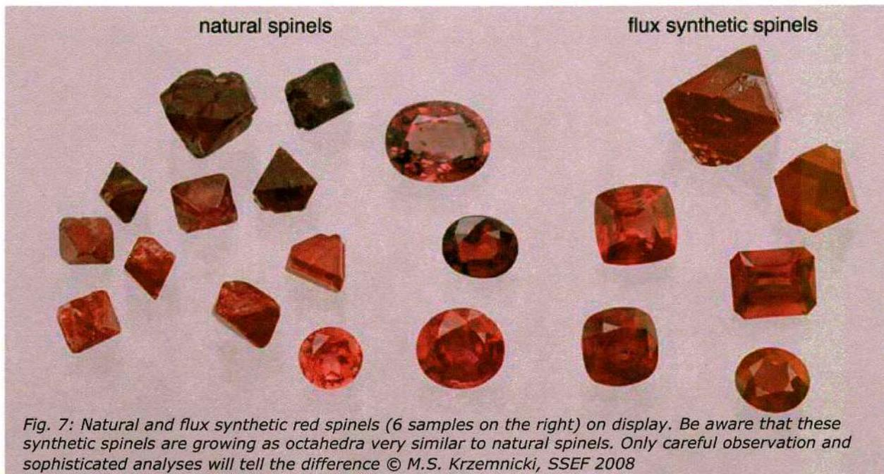
Fig. 7: Natural and flux synthetic red spinels (6 samples on the right) on display. Be aware that these synthetic spinels are growing as octahedra very similar to natural spinels. Only careful observation and sophisticated analyses will tell the difference © M.S. Krzemnicki, SSEF 2008
