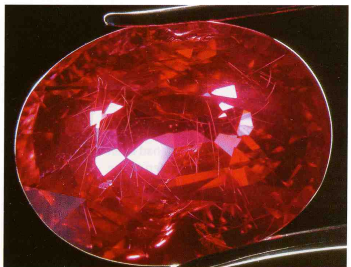
Ruby from Winza, Tanzania. Characteristic inclusions consist of fine bent fibers with a polycrystalline filling of probably secondary minerals. Photo © H.A. Hänni, SSEF Swiss Gemmological Institute.
