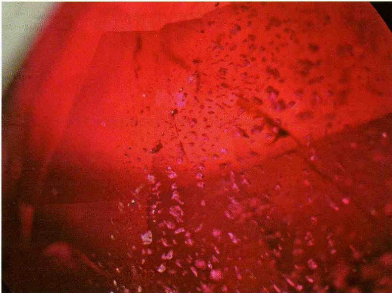
Ruby from Winza, Tanzania, with a healing fissure charged with multiphase inclusions. Photo © H.A. Hänni, SSEF Swiss Gemmological Institute.
