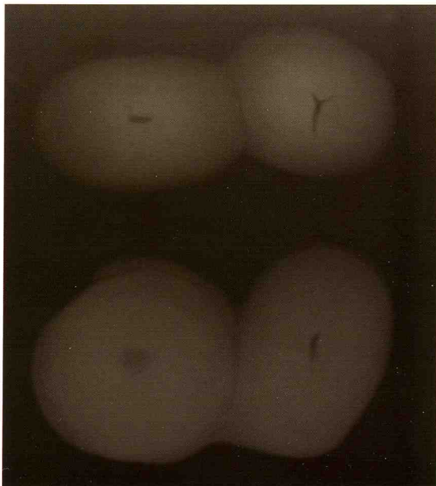
Figure 30. X-radiographs of the twinned pearl show features typical of beadless cultured pearls, especially the characteristic complex-shaped central cavity. Image by H. A. Hänni, © SSEF.
