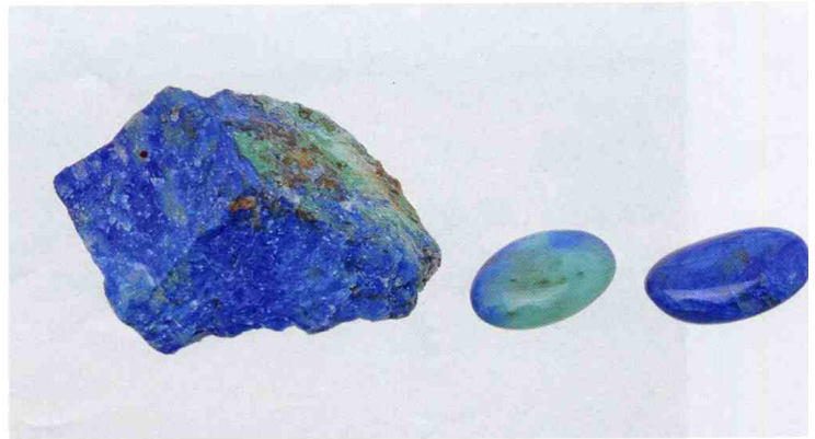
Figure 13. This feldspar-quartz-muscovite rock, sold in Tanzania, is naturally stained by secondary copper minerals. The blue color is due to azurite-filled veins, and the green is derived from malachite and chrysocolla. The cabochons are approximately 20 mm long. Photo by H. A. Hänni, © SSEF.
