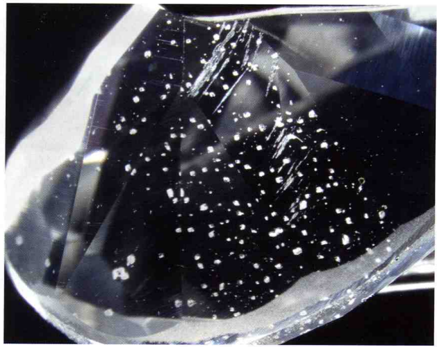
Figure 11. The forsterite contains a "fingerprint" composed of euhedral-to-subhedral inclusions. The linear features superimposed over the fingerprint are scratches. Photomicrograph by D. M. Kondo; field of view 7.2 mm.
