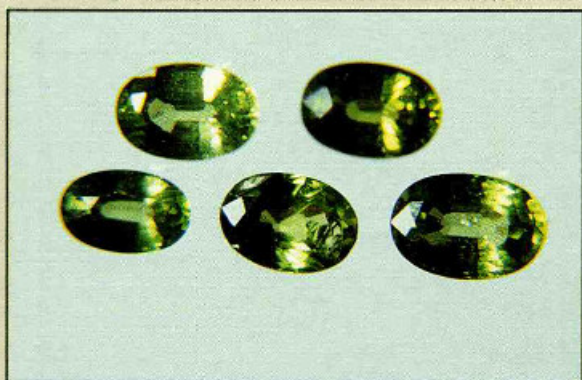
Figure 2: Faceted vanadium-bearing tourmalines from southern Madagascar. Weights of samples between 0.33 ct and 0.60 ct, the largest tourmaline (lower right) measures 4.4 x 6.5 mm.
