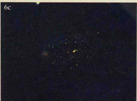
Figure 6: Healed feathers consisting of small cavities with multiphase filling (fluid with tiny magnesite crystals) are common in musgravites from Africa. (a) overview, the stone measures 5.5 × 7.5 mm; (b) in immersion, only tiny particles are common; (c) with crossed polarizers, the birefringent crystals are clearly visible. (b) and (c) magnified 70x.
