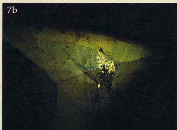
Figure 7: Musgravite with a healed fracture with two-phase filling (fluid and solid). The fluid channels are clearly visible in plane polarized light in immersion (a) and the birefringent crystals become visible using crossed polarizers (b). Magnified 70x.
