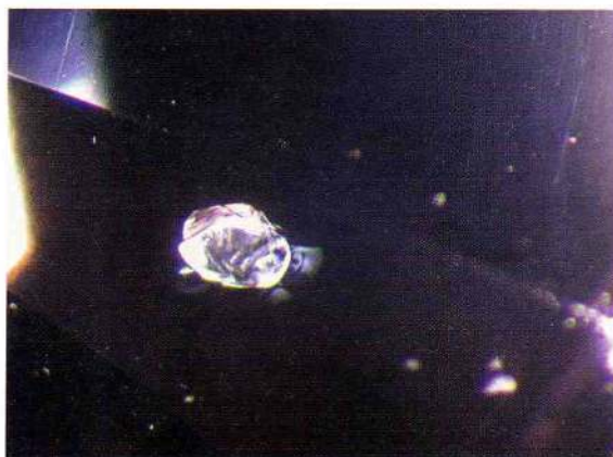
Figure 4: Rounded apatite inclusion in musgravite from Africa, magnified 80 \times .
