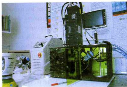
Fig. 6 LIBS system at the SSEF using a pulsed 266 nm Nd:YAG laser. © M.S. Krzemnicki, SSEF
