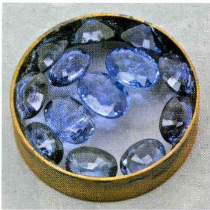
Fig. 8 Blue beryllium diffusion treated sapphires prepared in a sample holder for analyses with LA-ICP-MS. Under the microscope, most but not all of these stones show characteristic “diffusion clouds”. © M.S. Krzemiński, SSEF 2007
