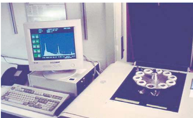
Fig. 6: Energy-dispersive X-ray fluorescence (ED-XRF) for chemical analysis. This instrument is used routinely in many gemological laboratories. © H.A. Hänni, SSEF
