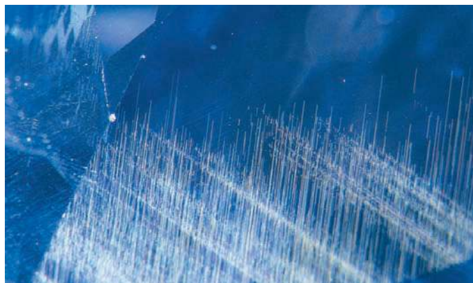
Fig 2: Fine and dense rutile needle aggregates are typically found in sapphires from Myanmar (Burma). Stones from Sri Lanka display long rutile needles, whereas sapphires from Kashmir show nearly no rutile inclusions. © H.A. Hänni, SSEF
