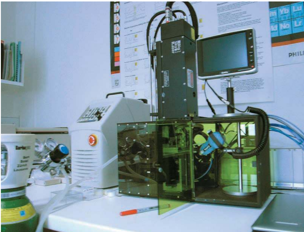
Fig. 8: SSEF Gem-LIBS. Chemical analysis of gemstones using a laser. © M.S. Krzemnicki, SSEF
