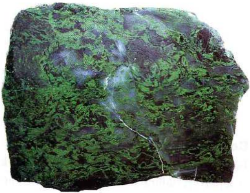
Fig. 5 A piece of Maw-Sit-Sit, a jade-related rock from Myanmar (Burma). The material contains at least eight different minerals and its visual aspect may change considerably according to the ratio of composing minerals. Photo © H.A. Hänni
