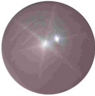
Figure 4: Rose quartz sphere (sample C) showing six-rayed asterism with a light spot at the intersection point of the arms of the star; the light spot at the right is the reflection of the fibre optic spot light used for illumination. This sphere weighs 158 grams and measures 4.9 cm in diameter.
