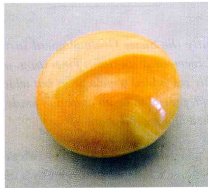
Fig. 1 The investigated specimen shows an orange colour similar to that of a melo pearl. A colourless transparent patch such as that seen on the top of the bead has never been reported on a melo pearl. The diameter of the bead is 23 mm. © M.S. Krzemnicki, SSEF 2006
