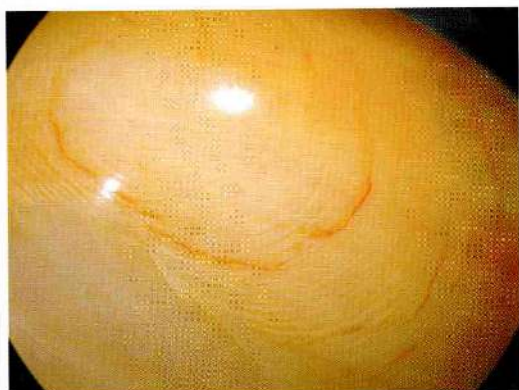
Fig. 3 Orange colour concentrations along cracks and “flames” on the specimen indicate dyeing. Further, a slightly curved horizontal layering, cross cutting the generally vertical flame structure, becomes visible under strong fibre optic light. This layering is interpreted as growth markings of the shell from which the bead has been made. © M.S. Krzennicki, SSEF 2006
