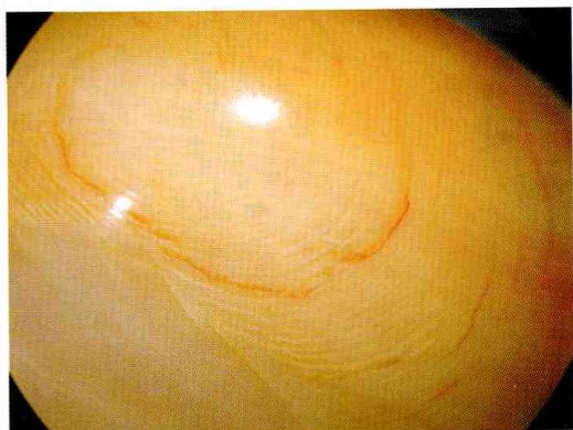
Fig. 3 Orange colour concentrations along cracks and “flames” on the specimen indicate dyeing. Further, a slightly curved horizontal layering, cross cutting the generally vertical flame structure, becomes visible under strong fibre optic light. This layering is interpreted as growth markings of the shell from which the bead has been made. © M.S. Krzemnicki, SSEF 2006
