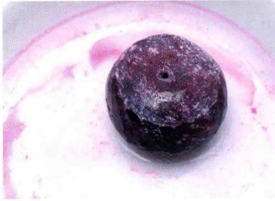
Fig. 3 Organic dyes are easily identified with a solvent like acetone. In this faceted bead all fractures were filled with red oil. Photo © H. A .Hänni, SSEF
