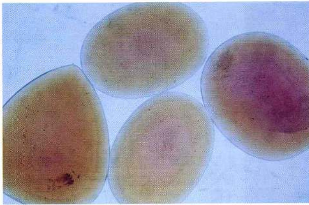
Fig. 4 Beryllium diffusion treated light pink sapphires with new yellow colour added in immersion showing yellow rim. Photo © H. A .Hänni, SSEF
