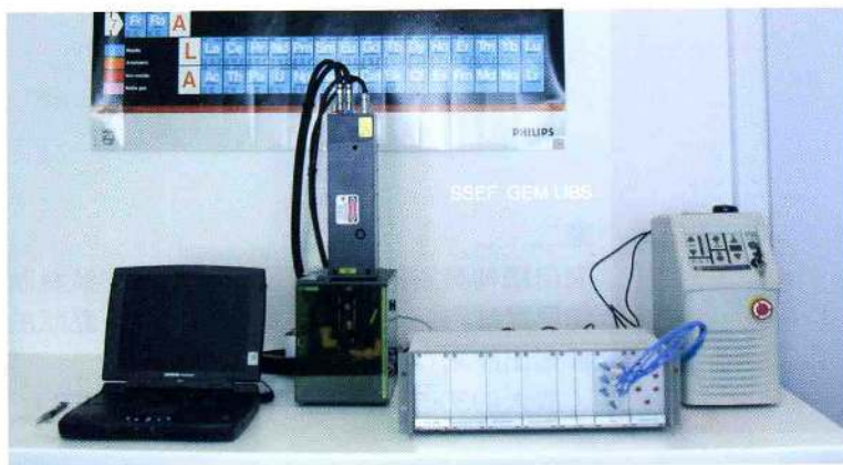
Fig. 5 The SSEF GemLIBS system to analyse low beryllium concentrations on cut stones. Analyses are usually performed on the girdle. Photo © H. A. Hänni, SSEF
