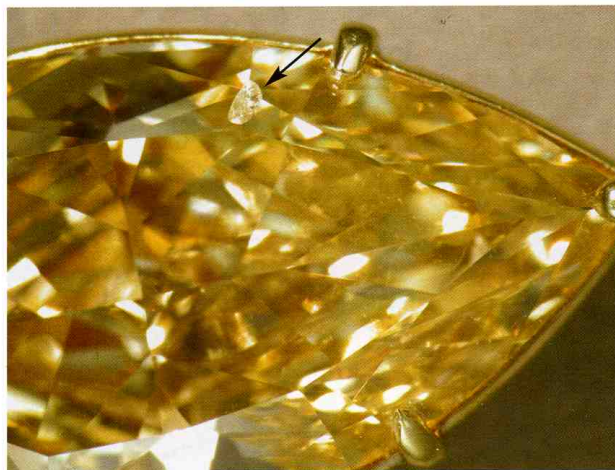
Figure 5. The chip (see arrow) on the crown of this yellow pear-shaped diamond appears to have been created by a misdirected shot from a laser soldering gun. A prong in the setting showed evidence of recent repair by laser soldering. A dark spot at the bottom of the pit was identified as graphite. Photo by H. A. Hänni, © SSEF.
