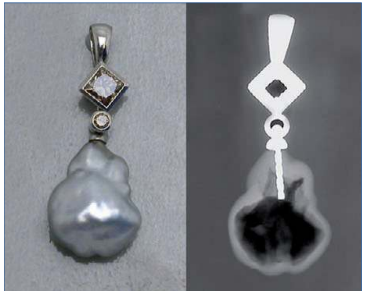
Figure 1: Beadless cultured Tahiti pearl – a so-called keshi – mounted as a pendant, with its radiograph showing a large irregular cavity (dark area). Length of the pearl 22 mm. Photo © H.A.Hänni, SSEF.
