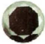
Right: Fig 2: Black diamond with colourless central zone and black rim due to many small black inclusions. © H.A. Hänni, SSEF 2005
