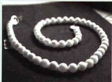
Figure 5: An Akoya cultured pearl necklace (freshwater nacre beads with saltwater nacre overgrowth) in room light, ready in the X-ray apparatus for a luminescence picture. Photo P. Giese © SSEF Swiss Gemmological Institute.
