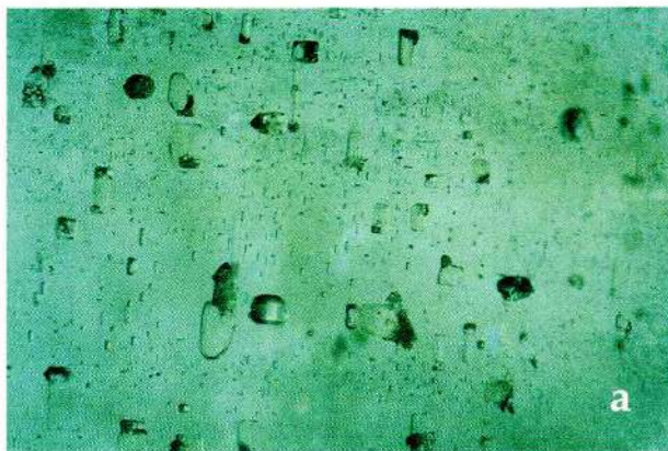
Figure 9: Emerald from Madagascar with six- and four-rayed asterism; short prismatic negative crystals and elongated channels parallel to the c -axis, view perpendicular to the c -axis. (a) 50 \times , (b) 100 \times .
