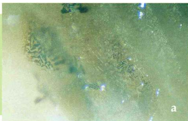
Figure 3: Bronze-brown six-rayed star beryl from Minas Gerais, Brazil; dense pattern of oriented ilmenite skeletal crystals, (a) view oblique to the c-axis, 100 \times , (b) view parallel to the c-axis, 100 \times .
