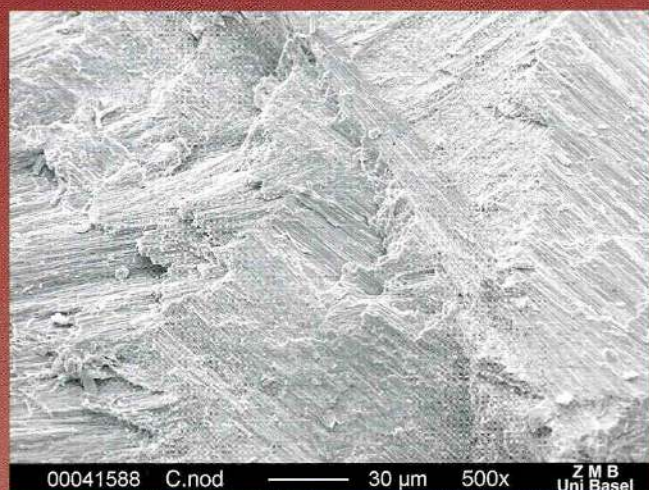
Figure 4: A broken section of a scallop shell shows that under the surface the bunches of fibres still have crossed orientations.
