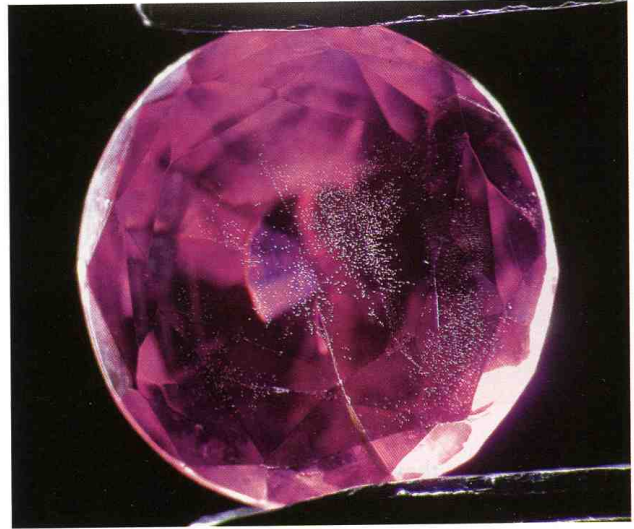
Figure 43. Gas bubbles appear to be radiating from the center of the color-zoned synthetic corundum (5.0–5.2 mm in diameter). Photomicrograph by H. A. Hänni, © SSEF.
