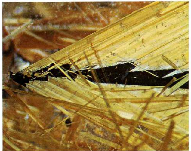
Figure 41. The orientation of the rutile inclusions, together with their dense, parallel formation and simultaneous reflectance create the appearance of moth wings, while the contrasting black hematite forms the "body." Photomicrograph by John I. Koivula; magnified 10x.
