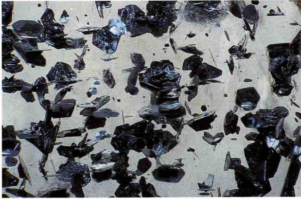
Figure 39. The molybdenite inclusions in the Chilean quartz display a characteristic lead-gray color and platy hexagonal form. Photomicrograph by John I. Koivula; magnified 10 \times .
