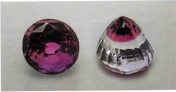
Figure 42. This 1.05 ct synthetic corundum appears uniformly purplish red when viewed face-up (left), while the color zoning is clearly visible from the side (right). Composite photo by H. A. Hänni, © SSEF.
