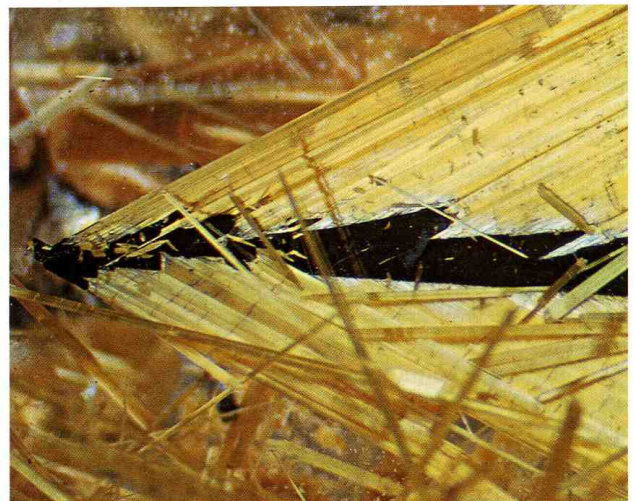
Figure 41. The orientation of the rutile inclusions, together with their dense, parallel formation and simultaneous reflectance create the appearance of moth wings, while the contrasting black hematite forms the "body." Photomicrograph by John I. Koivula; magnified 10 \times .
