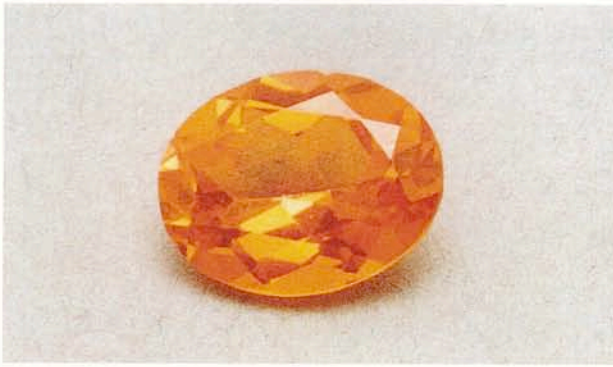
Figure 33. The orange color of this 2.95 ct topaz is caused by a thin coating of synthetic hematite applied to the pavilion. Photo by Michael S. Krzemnicki; © SSEF Swiss Gemmological Institute.
