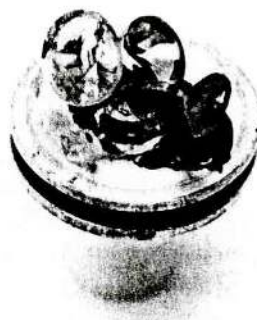
Fig. 3: Treated yellow & orange sapphires, after treatment, still bearing glassy flux layer
